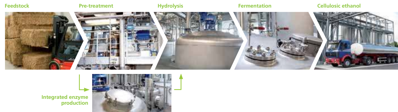
The sunliquid® process for the production of cellulosic ethanol from agricultural residues
